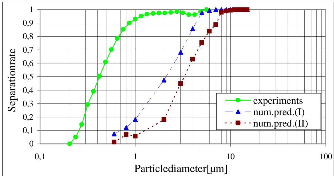
Comparison of experimentally and numerically predicted particle separation rates for ZS18 with  $h_{ac} = 18.7 \text{ mm}$ ,  $u_F = 25.0 \text{ m/s}$ .
