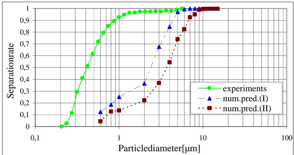
Comparison of particle separation rates for ZS30 with  $h_{ac} = 30.0 \text{ mm}$ ,  $u_F = 25.0 \text{ m/s}$  (I –  $\rho_P = 2700.0 \text{ kg/m}^3$ , II –  $\rho_P = 1000.0 \text{ kg/m}^3$ ).
