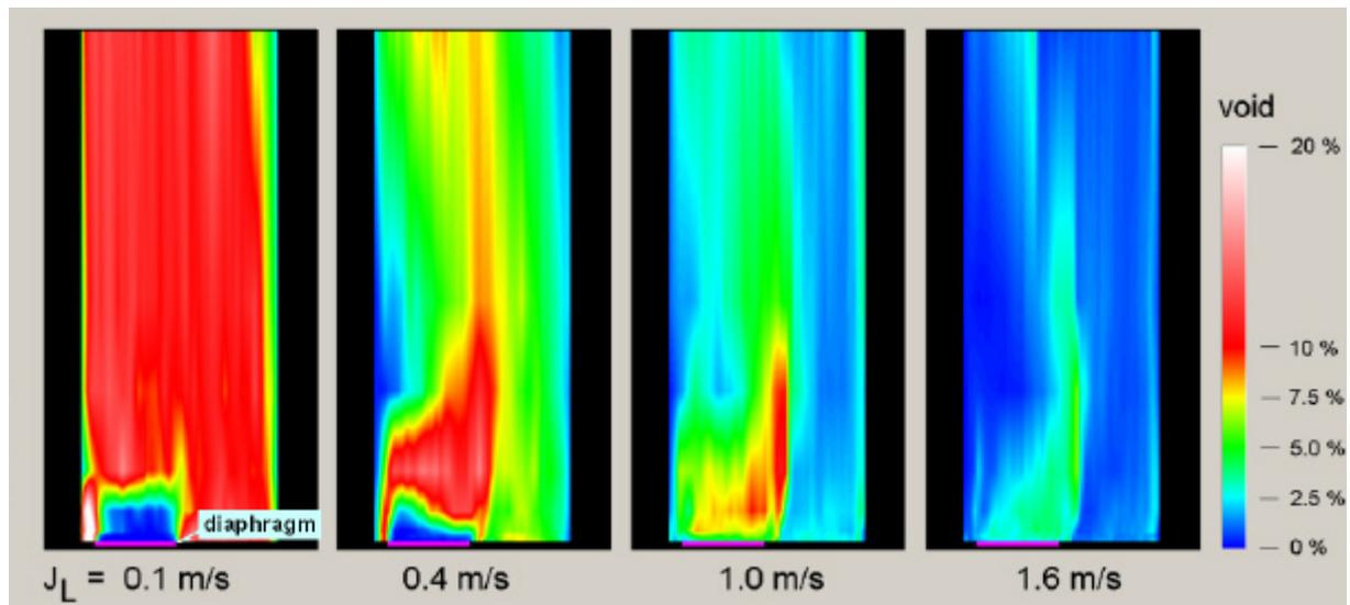
Fig. 6: Change of void fraction profiles downstream of the diaphragm at  $J_G = 0.037$  m/s with a variation of the superficial liquid velocity  $J_L$ .
