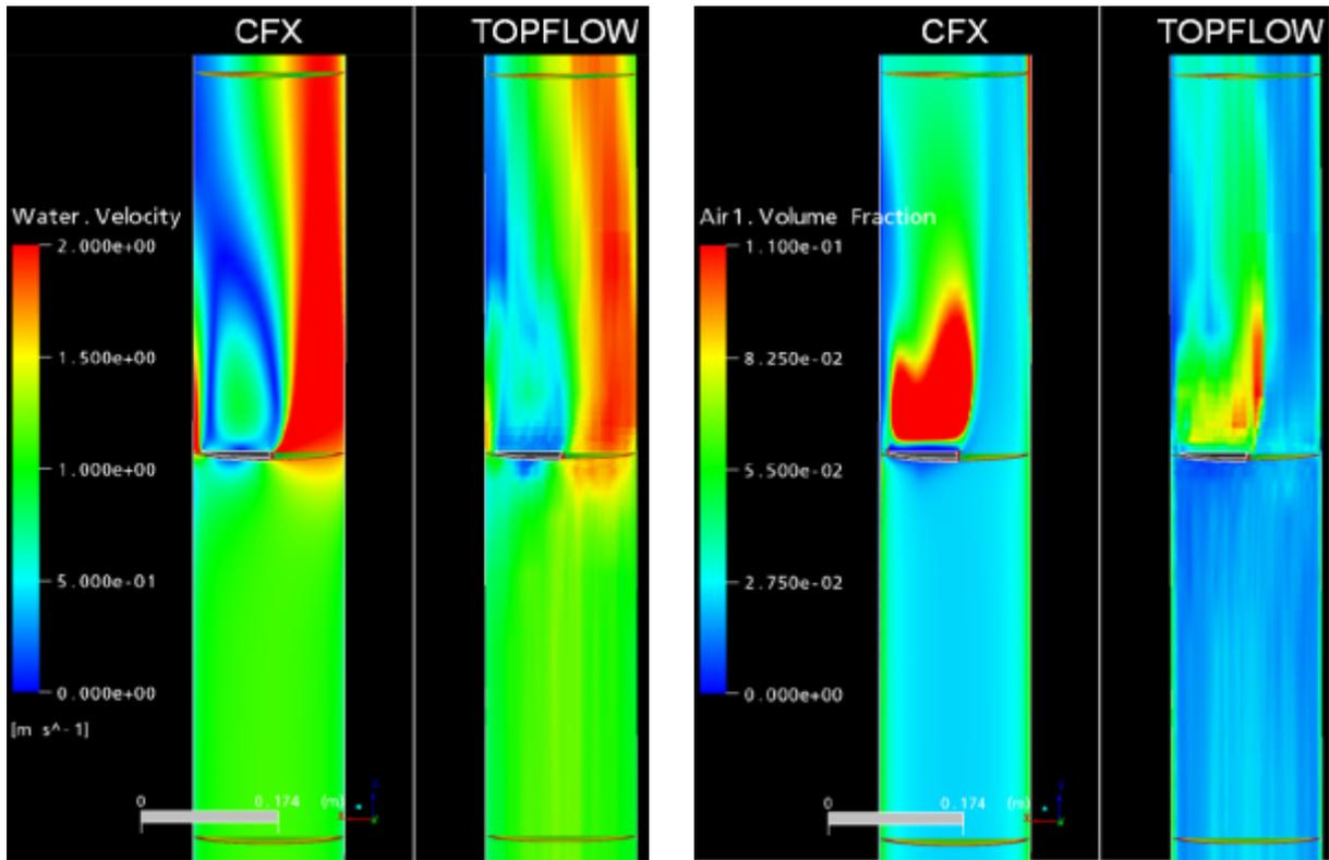
Fig. 8: Comparison between experiment and CFX pre-test calculation for the absolute water velocities (left) and the gas volume fraction distribution (right) for the region from 0.5 m upstream to 0.5 m downstream the obstacle; air-water test at  $J_L=1$  m/s and  $J_G=0.037$  m/s.
