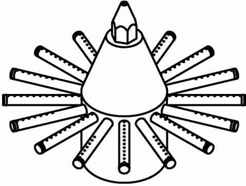
Fig. 3: Gas injection head
