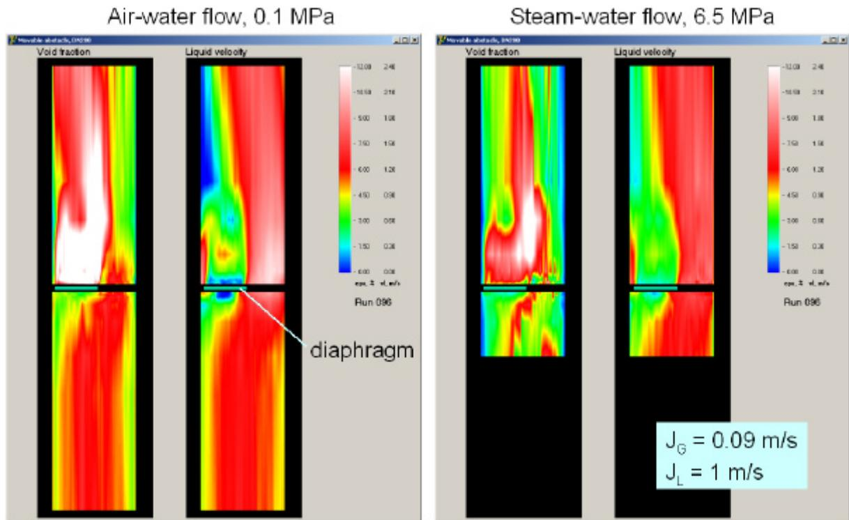
Fig. 7: Void fraction and liquid velocity profiles in an air-water and a steam-water test at identical superficial gas and liquid velocities.
