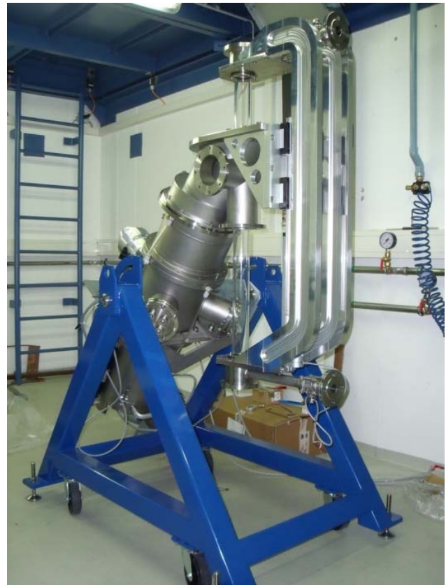
Figure 11: Working principle of the ultrafast CT scanner ROFEX (left) and photography of the special designed system comprising the bundle test section
